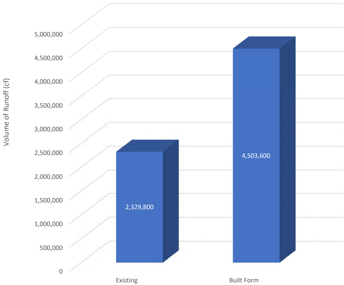
Figure 12 Volume of Runoff 2 YR-24 HR Rainstorm Event Existing Single family to Corridor 3, 4, and 6 Built Forms
